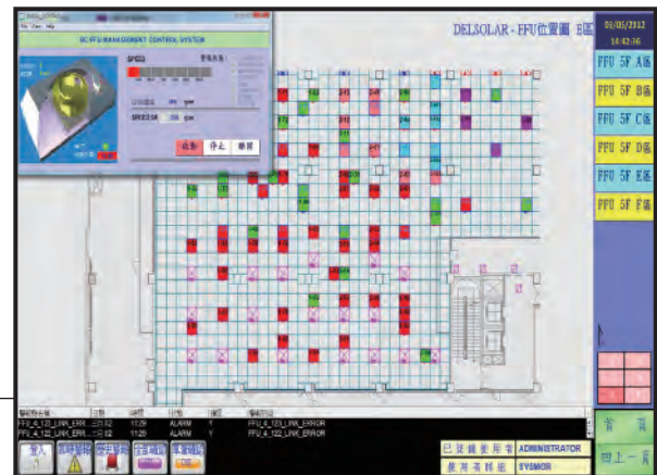
中文INTOUCH 圖控軟體，與廠務監控系統整合容易 INTOUCH software applicable for the monitoring and control system, enable the integration to FMS.
